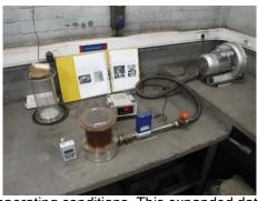
lab-scale permeability measuring device available. The goal of the master thesis is to draw clear correlations between the sinter mix properties, its permeability and the resulting productivity. In a second step, guidelines are to be defined which should allow the operating staff to exploit the sinter plant even more.
